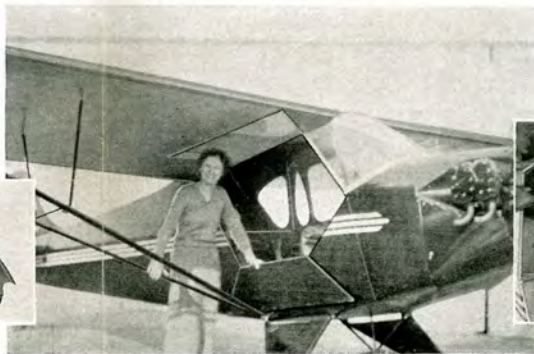
In the New "CUB" Cabin two nicely upholstered seats are placed in tandem. Dual controls allow the ship to be operated from either seat by student, passenger or pilot. This makes the New "CUB" an ideal training plane and assures an additional degree of safety. Entrance to the Cabin is easy, even with heavy clothing and parachute, as the wide door opens up under the wing.
