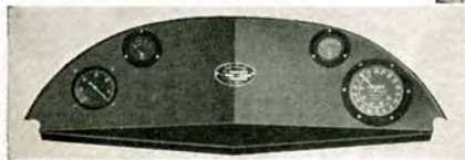
The New "CUB" Instrument Panel complete with altimeter, tachometer and oil pressure gauge shows how the ship is performing. The temperature gauge and gasoline gauge may be read at a glance.
